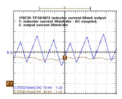
'stable' operation. Inductor current is AC-coupled. L2 is 33uH sliding-mode choke.
